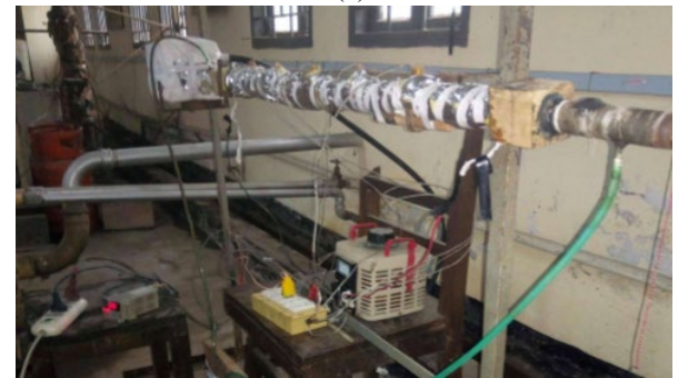
FIGURE 1. (a) Cross sectional view of the designed tube with inserts at 45° orientation (b) 6 inserts layout at 45° orientations (c) Photograph of copper tube after the thermocouple brazing (d) Photograph of the experimental setup
